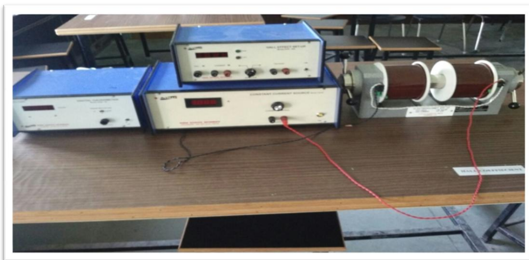
Magnetic Field Sensing Probes and electromagnet based Hall effect setup in physics lab
