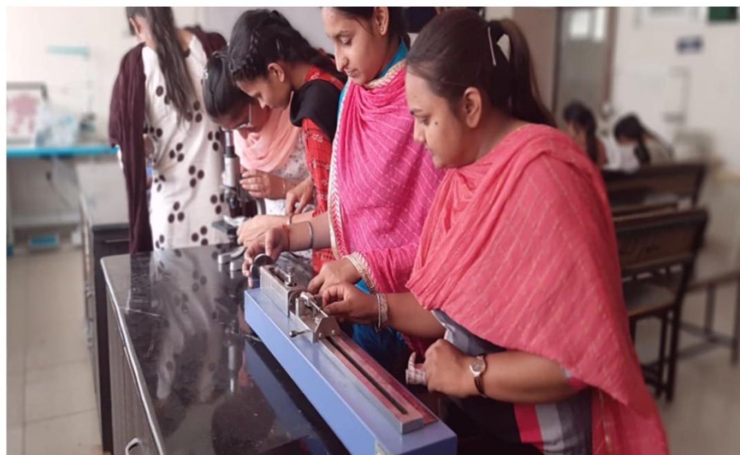
Testing yarns on Twist Tester by Students of Fashion Technology
